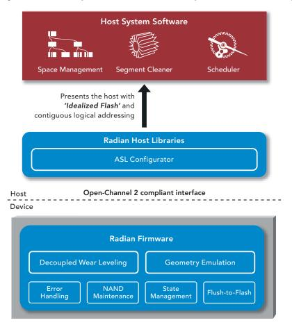
Radian brings some of its innovative Cooperative Flash Management (CFM) technology into its unique SSD implementation that has an Open-Channel 2 compliant interface:
