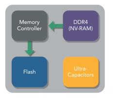
transferred to persistent NAND memory by the Flushto-Flash firmware. The overall Flush-to-Flash system and underlying NAND array are based on a fault tolerant architecture, utilizing transactional semantics and ACID design principles.
