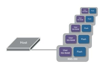
The example below illustrates how the RMS-350 enables a host to write data into its on-board NV-RAM, then issue a single Delegated Move command to transfer the data from NV-RAM to local Flash storage.
