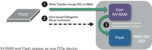
The User NV-RAM and Flash appear as one PCIe device, but as two distinct block devices.
